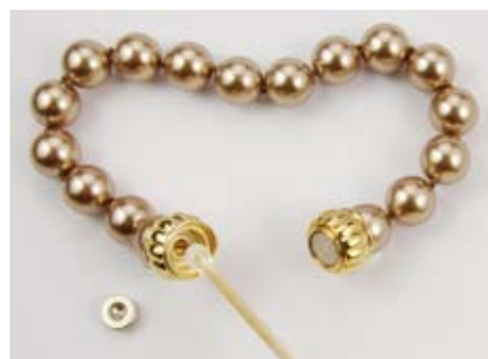
Epoxy holds even strong magnets in their clasp halves.
